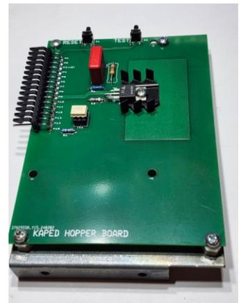
SNAP THE NEW BOARD WITH MOUNTING STUDS INSTALLED ONTO THE ORIGINAL BRACKET.
