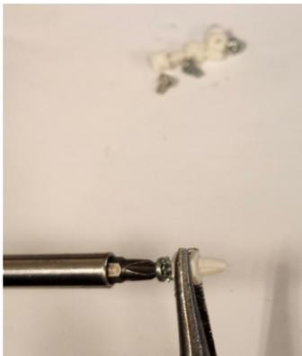
MOUNT THEM ONTO THE BACK OF THE NEW BOARD IN THE HOLES SEEN IN THE PHOTO.
